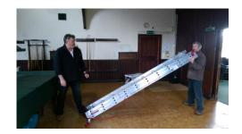
Undo the clips at the base and separate the 2 widest ladder sections until the tapes are taught. Fix in place the bracket that holds the 2 lower sections apart ensuring it is properly attached.
